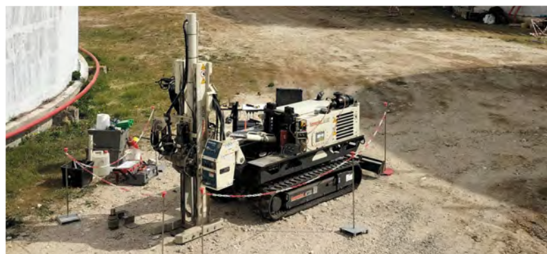
Geoprobe 6712DT® is equipment for sampling different environmental matrices.
